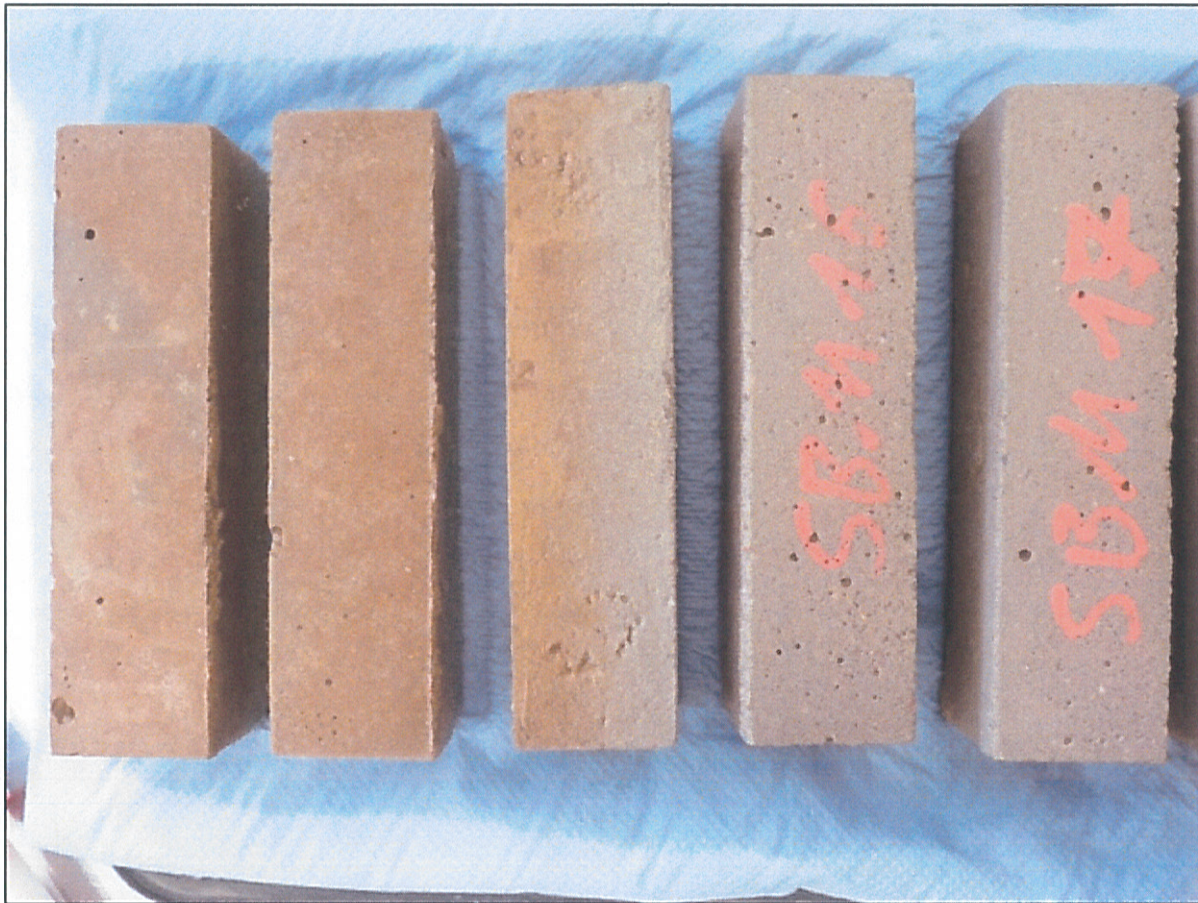
Figure 6: Discoloration of the SBM prisms after the acid exposure
